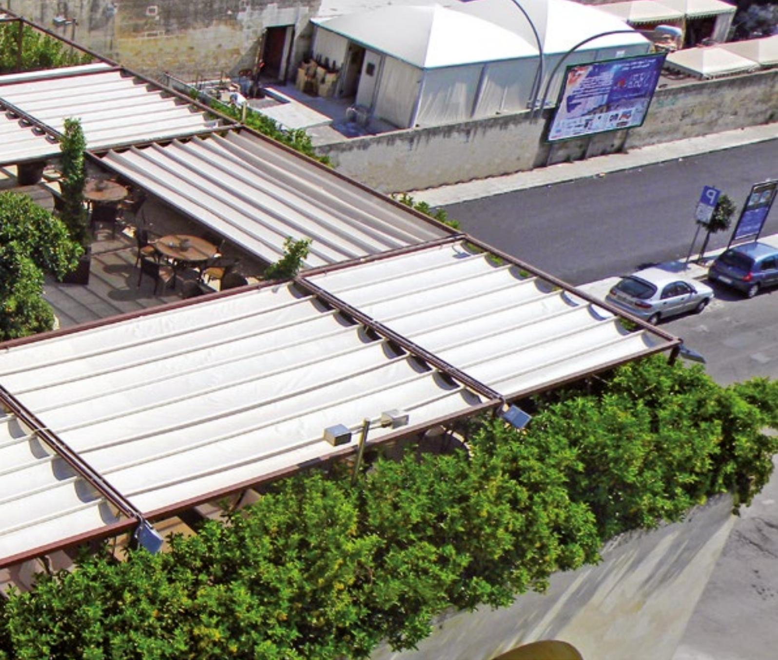
**Beach System:** Manual sliding roof system with aluminum frame and fire retardant PVC roof.
